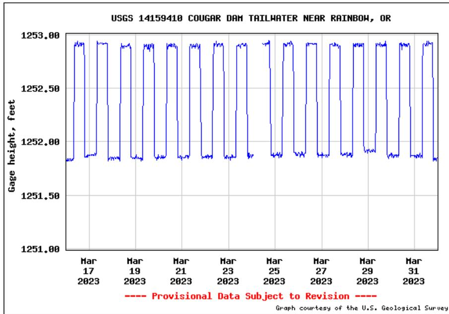
Figure 30. Gage Height (feet); below Cougar Dam, South Fork McKenzie River
